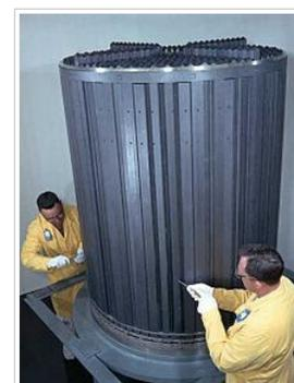
The core of the Molten Salt Reactor Experiment
