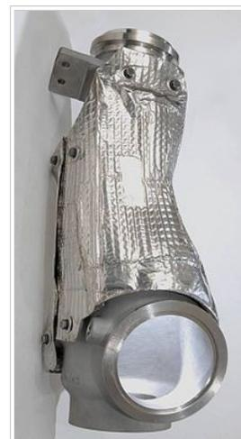
A particulate filter housing for a regenerative burner made of CF8C Plus stainless steel
